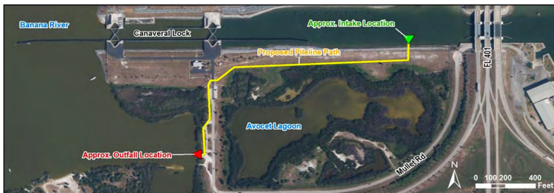
Figure: Aerial view of Canaveral Locks with proposed pump intake and outfall locations and pipe route. Pilot design is preliminary and subject to change.
